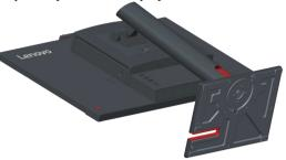
Step 3: Remove the base and stand from the monitor.
