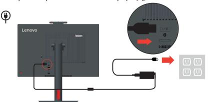
**Note:** When installing the computer to the TIO monitor for AIO mode, ensure you use the power adapter that comes with the computer when computer power adapter large than 90W, otherwise please use TIO power adapter.
