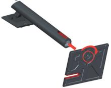
3. Insert the two metal tabs on the stand into the corresponding holes on the rear of the monitor. Then, pivot the stand downward until it clicks into position.
