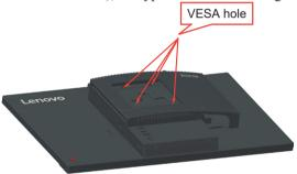
Step 5: Attach the LCD display to the wall, and follow the instructions in the wall-mounting kit.
