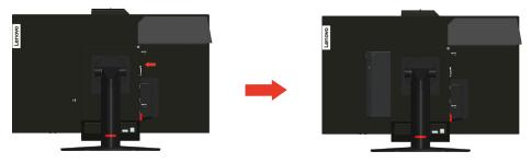
3. Pull the computer out of the computer bay. Then, pivot the cable cover as shown to the closed position.
