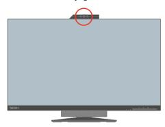
Slide the camera shutter open or close to enable/disable the camera.
