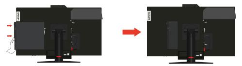
3. Press the computer from the front until it completely snaps into position.
